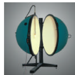
Option Digilumen to measure luminous flux with integrating sphere
