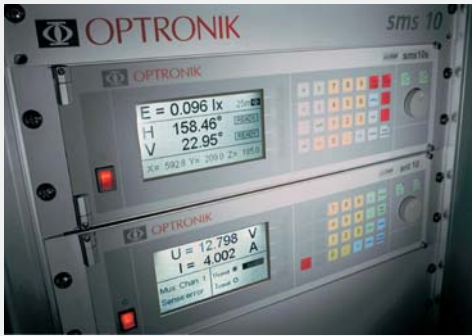
SMS10s Control and Photometer Unit with SNT10 DC Power Supply
