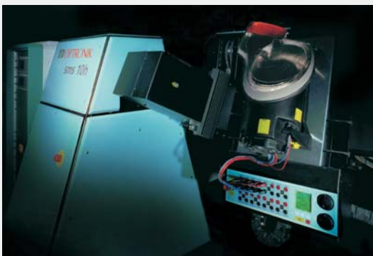
SMS10H high Speed scanning Goniophotometer equipped with Vv10dsp Preamplifiers
